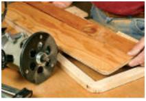
The secondary template the author is holding was used to shape the edges of the infill frame that was assembled with half-lap joints. The template was screwed in place with about 1/2" of the frame exposed on three sides. Then it was a simple matter of routing around the template to trim the frame to exact size.
