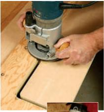
Use your master templates (the author used a good size Forstner bit to form the corners) to form the cutouts in the desktop (far left). The templates will guide a router fitted with a 3/4"
