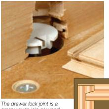
The drawer lock joint is a great way to join plywood drawer sides because it covers the plywood strata as shown in the drawing at left. The author also cut the groove for the drawer bottoms using the
