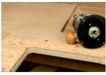
The final, trimmed edge (on the inside of the three-sided infill frame) is produced using the master template and the same router, guide and bit combination that made the initial cutout.
