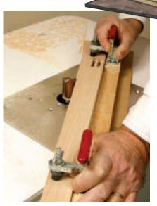
Attach fences to the leg template, and mount a couple of toggle clamps on them to secure the leg blank. Band-saw off the majority of the waste, then template-rout the leg flush using a bearing-guided bit.
