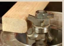
With its center bearing and a little fine adjustment, this bit forms perfectly sized hardwood edging with plenty of glue surface.
