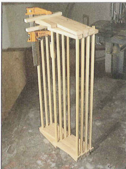
Photo B: Close up the rack and clamp together
