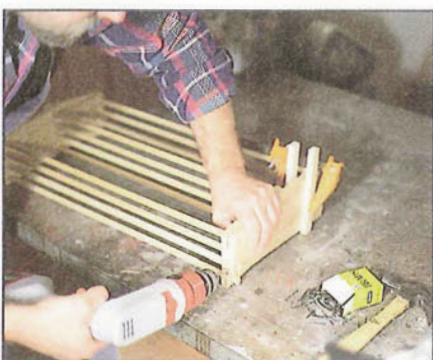
Photo C: Lay the rack down and brad the outside stretchers
