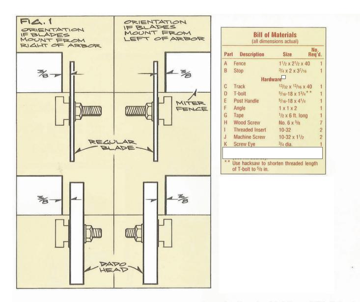
in. block for the stop (B). We used oak for our fence and maple for the stop. As with any project that requires hardware, we suggest you have the hardware on hand before starting.
